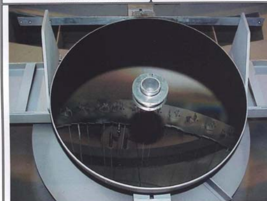
Realuminized – Hanging in Tank
